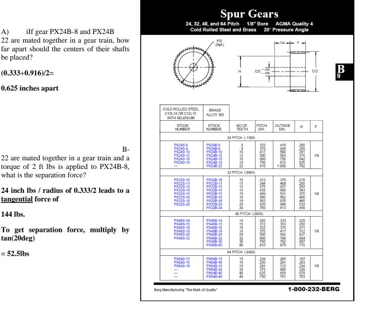
C) If gear PX 24B-8 and PX24B-22 are mated together 0.02 inches farther apart than you determined in part A, what are the primary consequences? Would your answer to part B change and if so would it rise or fall?
