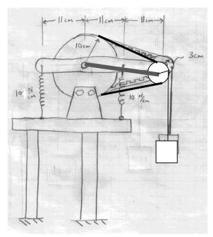
Due to the small angles and generous  $\pm 20\%$ allowance for our estimate, we can linearize. We have a motion of the weight due to two factors: Rotation of the arm => 0.1 rad\*24\*cm=2.4 cm downward
